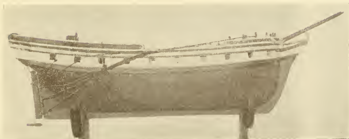
SHIP "ULYSSES" (2d) OF SALEM Model made in 1804 by Capt. William Mugford to illustrate his temporary rudder.
